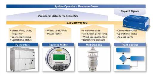
T1-S Gateway exchanges status data and dispatch signals between CAISO and intelligent devices to facilitate compliance, support performance monitoring and ensure operational excellence.
