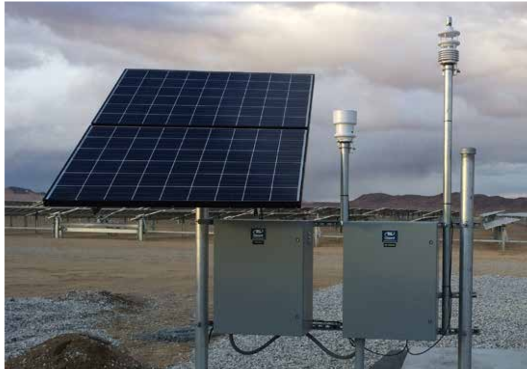
In addition to the standard measures, this meteorological station monitors precipitation. This station also includes a battery backup and PV-based recharging system to provide autonomous operation and ongoing data capture in case of power disruption.
