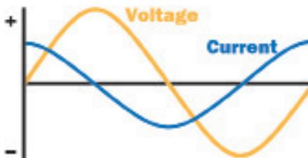
Fixed shunt capacitors and reactors can be used to shift the dynamic reactive capability of a generating facility to a lagging or leading power factor respectively. These static reactive devices can be used to supplement the total reactive capability of a generating facility. If there is insufficient dynamic reactive power availability from other devices at the facility, SVCs or STATCOMs can be used to increase the total dynamic reactive power capability of the facility.
